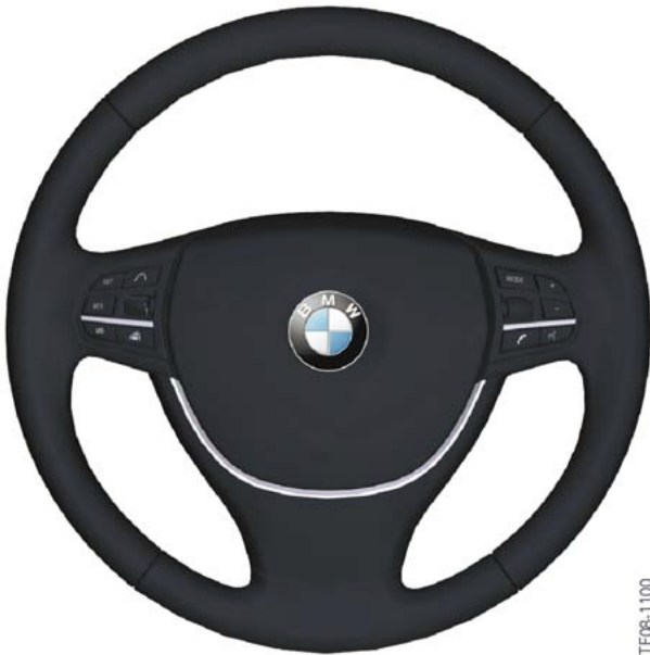
F10 Steering wheel with driver's airbag
